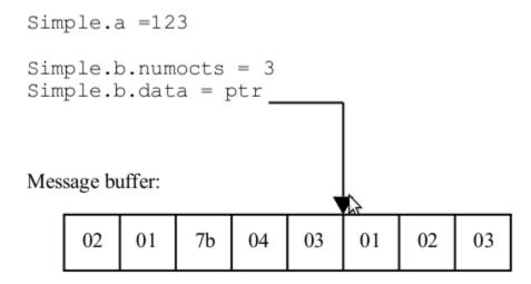
The pointer stored in the data structure points directly at data in the message buffer. No memory allocation or copy is done.
