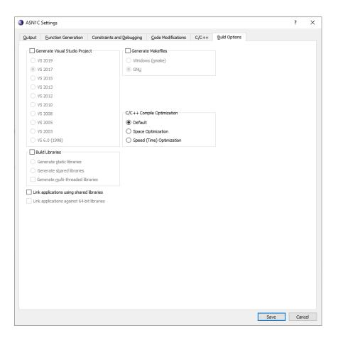
A makefile can be generated in either Windows or GNU format. For Windows, a Visual Studio project can also be generated. Under the Build Libraries section, which generates the build script to build a library rather than an executable, the desired variety of library can be selected.
