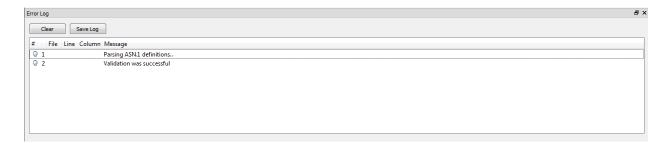
In many cases, an error is associated with a particular portion of the schema being compiled. Click on an error to open the schema editor at the location in which the error occurred. If more than one error is reported, clicking Next Error and Previous Error in the toolbar moves the Editor window to the part of the schema where the next or previous error occurred.
