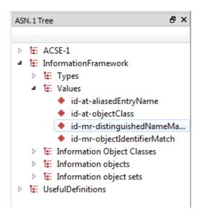
At the top level of the tree, the modules of the schema are shown. Each of these modules can be expanded to reveal branches for the types, values, information objects, etc. defined within. Click on any node of the tree to show the relevant ASN.1 definition in a built-in browser in the Editor window.
