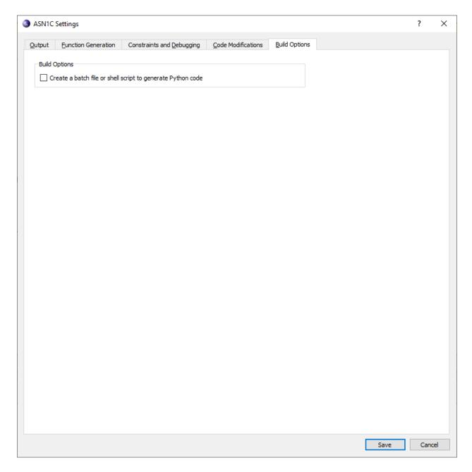
For Python, ASN1C can create a batch file (Windows) or shell script (non-Windows) that generates the Python code as set up by the GUI settings.
