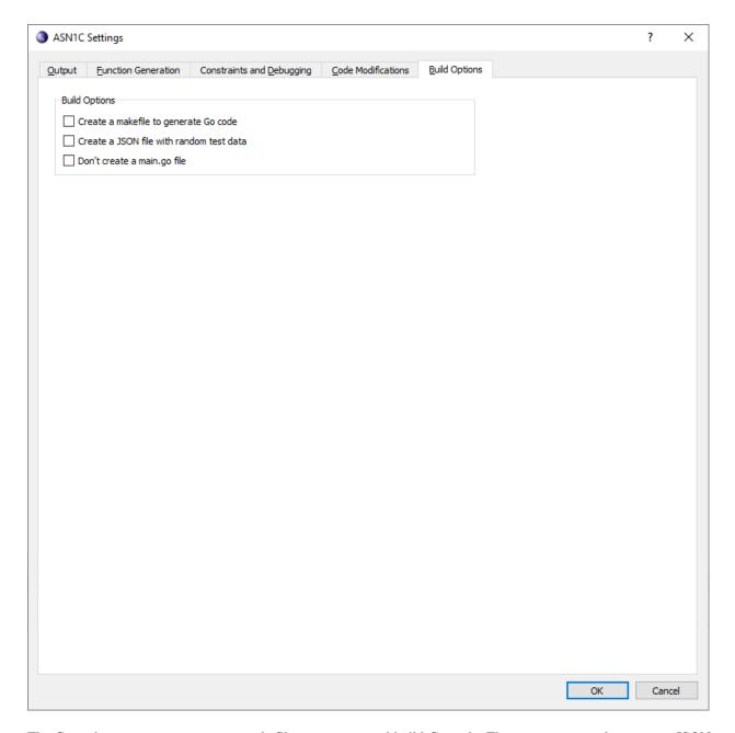
The Go code generator can create a makefile to generate and build Go code. The generator can also create a JSON file with random test data. Additionally, an option for the generator not to create a main.go file (for instance, if there already is one that has been modified) is available.
