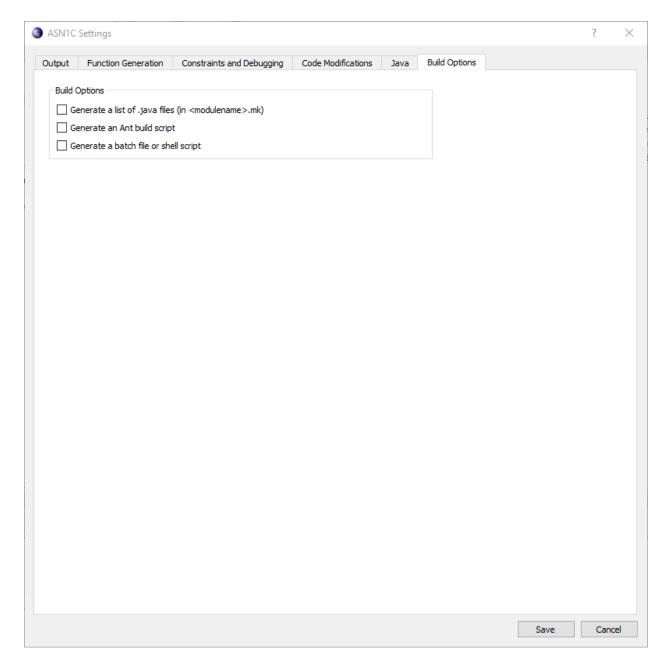
$Like \ C\#, Java\ can\ also\ provide\ a\ *.mk\ generated\ file\ list,\ as\ well\ as\ an\ Ant\ build\ script\ and\ a\ batch\ or\ shell\ script.$
