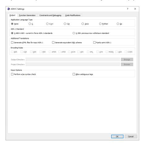
The Output tab is displayed by default. In the Application Language Type section, select C. In the Encoding Rules section, select BER. Finally, in the Output Directory text box, enter or browse to the location where the generated files should be saved. When finished defining the project settings, click OK. These settings can be changed at any time by selecting Project > Project Settings from the menu.
