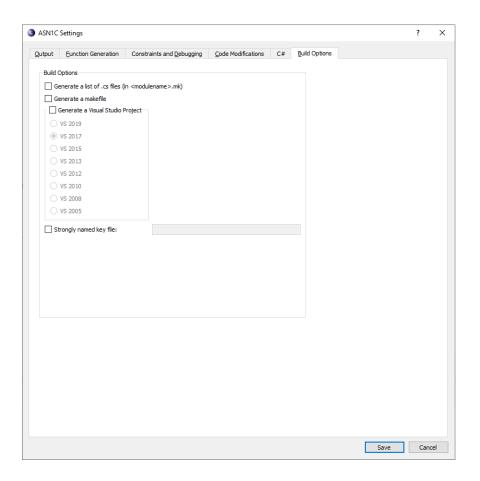
For C#, a makefile or Visual Studio project can be created, optionally including a \*.mk file listing the files generated. An option to specify a strongly named key file is also available.
